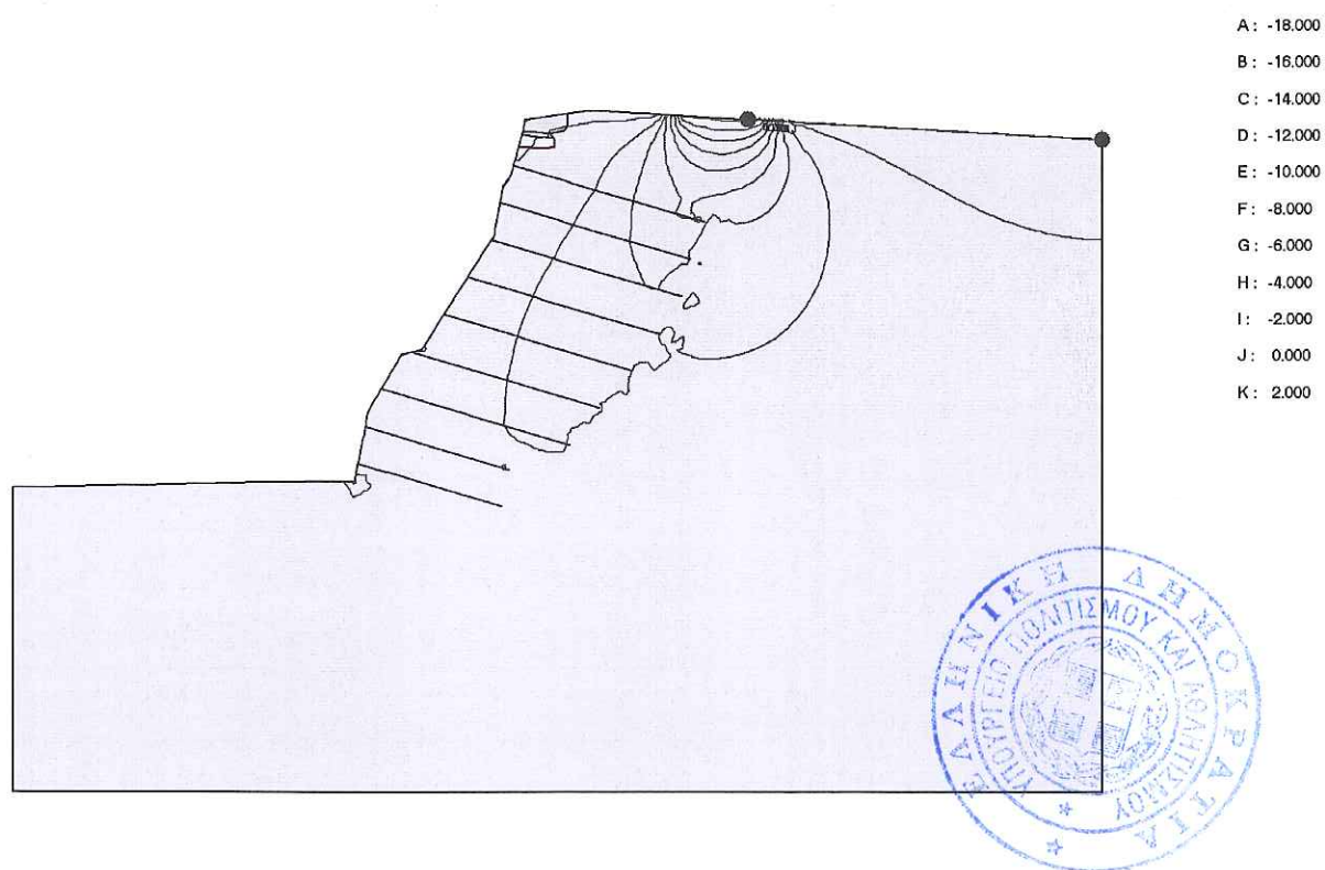
Fig. 23 Plot of total stresses (mean contours) - step no: 4 - ( phase: 3 )
